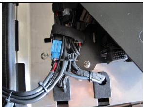
If a mobile radio is used, the receiver will need to be relocated to the LH saddlebag, not only for reasons of space, but also weight distribution. The FMS Accessories Radio Reciever Relocation kit includes a special mounting bracket along with radio power cable extension complete with BMW connectors, grommets and all needed hardware.
