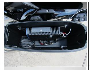
Attach the Brother PocketJet printer to the printer housing using the Velcro tabs provided. If battery access is needed, you may wish to carefully cut the Velcro strips as they cross over to the battery on the printer. The Velcro strips keep the printer not only in place while riding, but also from rocking or "torqueing" when it feeds paper, so the Velcro needs to span the full width of the printer.
